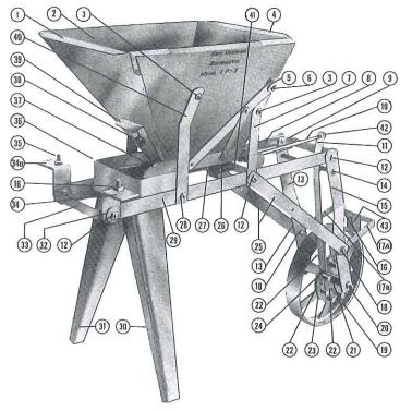
A tractor mounted Side Dressing Distributor for applying fertilizer to two rows at one time during the normal cultivation procedure. The unit can be adjusted to distribute fertilizer at any normal rate per acre and can be used on any normal width rows.
